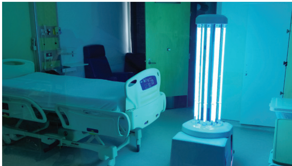
Sterilizing a room is a labour-intensive process taking hours, but the UV-disinfection robot can do it in a fraction of the time, sparing cleaning staff the risk of infection
