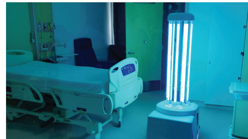
Sterilizing a room is a labour-intensive process taking hours, but the UV-disinfection robot can do it in a fraction of the time, sparing cleaning staff the risk of infection
